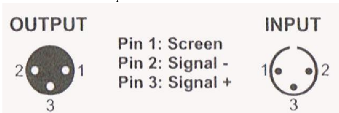
Three pin (Canon) DMX512 connector
