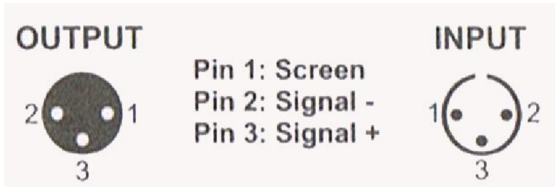
Three pin (Canon) DMX512 connector
