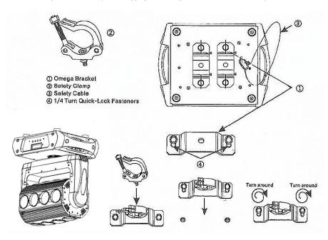
Regardless of the rigging option you choose for our LED Fantastic Roller , always be sure to secure your fixture with a safety cable. The fixture provides a built-in rigging point for a safety cable on the hanging bracket as illustrated above. Be sure to only use the designated rigging point for the safety cable and never secure a safety cable to a carrying handle.
